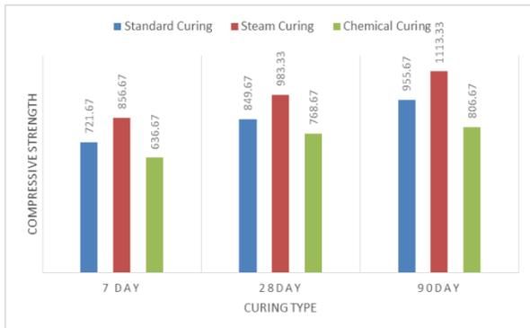
**Figure 3: Compressive strength results for mix MS0 under different type of curing**
