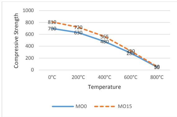
**Figure 8: Development compressive strength results for metakaolin concrete under different degrees of temperatures and ordinary Portland cement mixes at (28 Days)**
