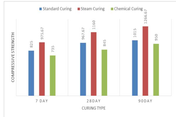
**Figure 4: Compressive strength results for mix MS15 under different type of curing**
