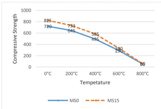
**Figure 9: Development compressive strength results for metakaolin concrete under different degrees of temperatures and Sulphate resistance cement mixes at (28 Days)**
