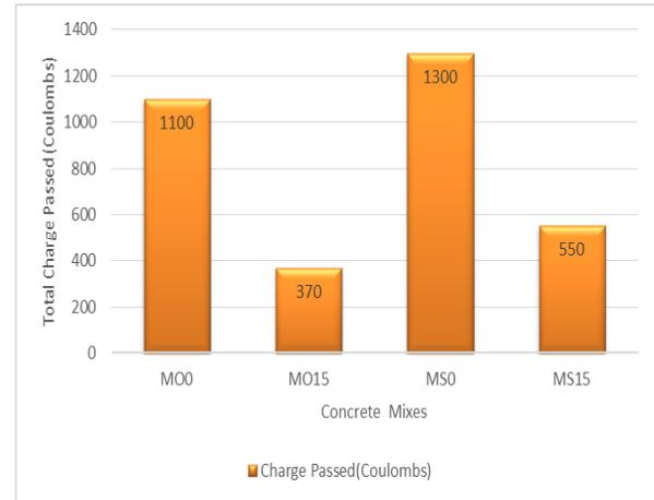
**Figure 7: Development the chloride penetration test results for Mix contains metakaolin and different types of cement at (28 Days)**
