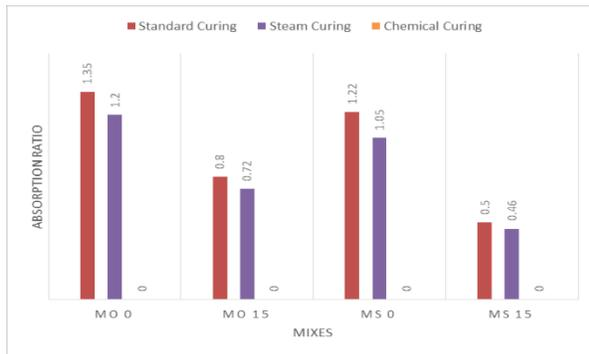
**Figure 6: Development comparison between absorption ratios for Mix contains metakaolin under different type of curing at (28 Days)**
