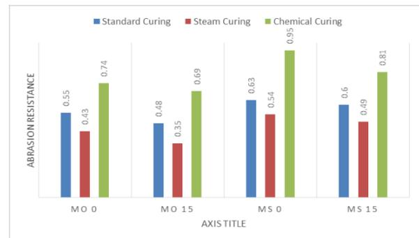
**Figure 5: Development comparison between abrasion resistances for Mix contains metakaolin under different type of curing at (28 Days)**
