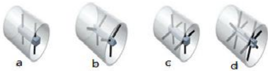
Figure 2: In-pipe robotic structure form: a) single-plane form. b) 3-plane form. c) 4-plane form. d) 6-plane form, reproduced from [14]
