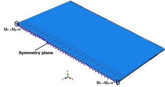
Figure 5: Mechanical boundary conditions
