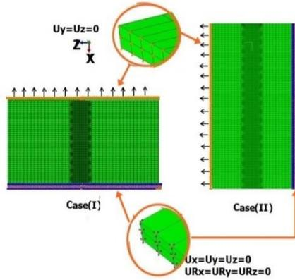
Figure 8: Boundary conditions and loading for the through-cracked thin plate.
