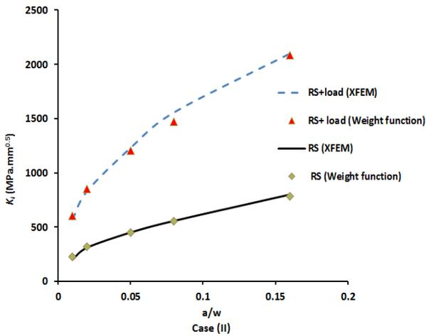
Figure 17: The values of  $K_I$  subject to RS and combination of RS and external stress in Case (II).
