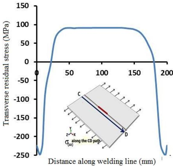
Figure 14: Transverse residual stress  $\sigma_{zz}$  (MPa) along the CD path.
