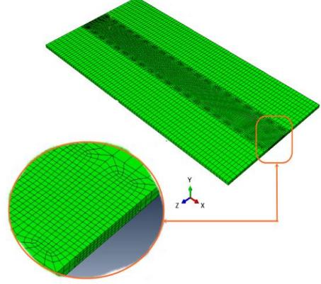
Figure 3: Mesh details for the finite element model of a butt-welded plate.
