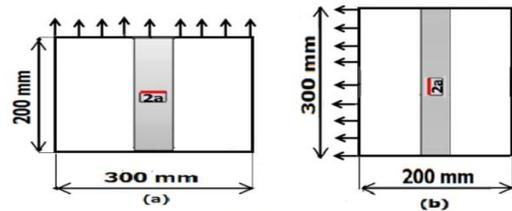
Figure 6: Loading and dimensions for the cracked joints, where  $2a$  represents the crack: a) case (I): transverse crack, and b) case (II): longitudinal crack.
