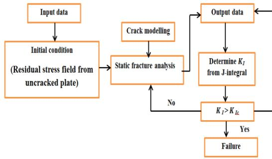
Figure 7: Flow chart for the 3D crack analysis.
