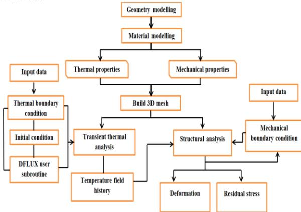
Figure 2: Flow chart for 3D thermo-mechanical finite element analysis.
