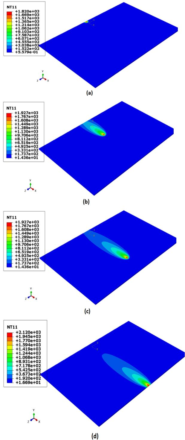
Figure 9: Temperature contour of the plane without cracks in the heating process: (a)  $t = 1.4$  s, (b)  $t = 30$  s, (c)  $t = 60$  s, (d) 79.4 s;  $t$  denotes the time after the heating process is started.
