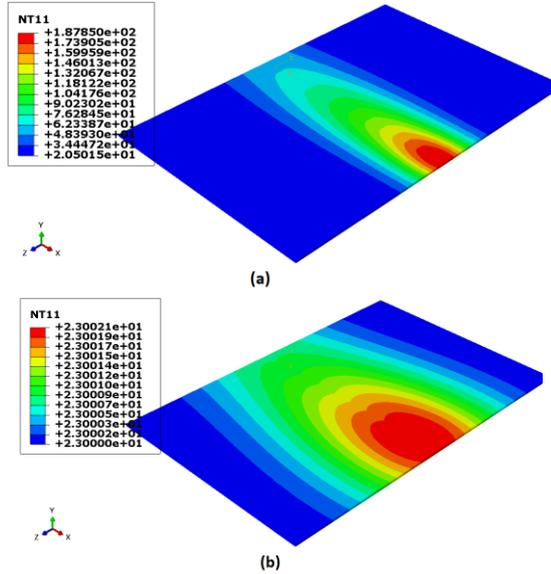
**Figure 10: Temperature contour of the plane during the cooling process: (a)  $t = 119.5$  s and (b)  $t = 1500$  s;  $t$  denotes the time after the completion of the welding process.**
