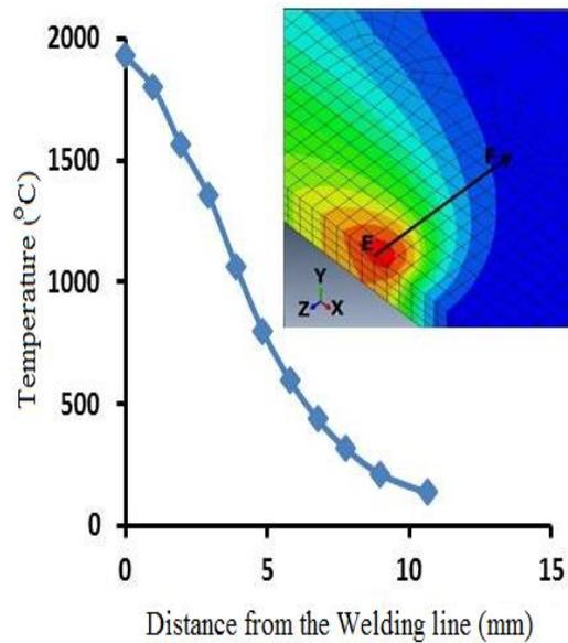
**Figure 12: Temperature distribution along the EF path.**
