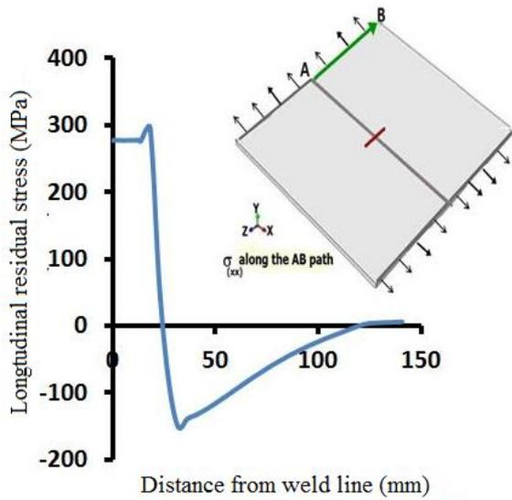
Figure 13: Longitudinal residual stress  $\sigma_{xx}$  (MPa) along the AB path.
