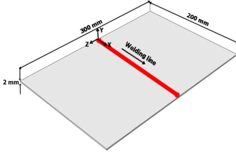
Figure 1: Dimensions of the geometrical model.
