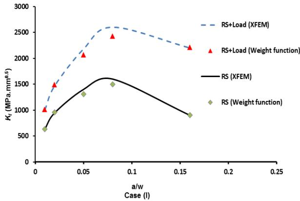
Figure 16: The values of  $K_I$  subject to RS and combination of RS and external stress in Case (I).
