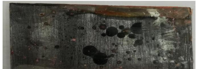
Figure (12): Blank epoxy coated sample after 42 days of Acetone exposure
