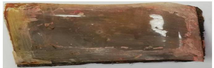
Figure (14): Blank epoxy coated sample after 6 days of HCl exposure
