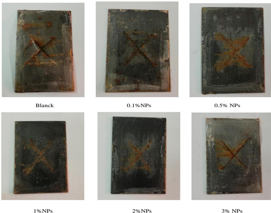
Figure (5): Salt spray images for 1% Chitosan with different concentrations of NPs
