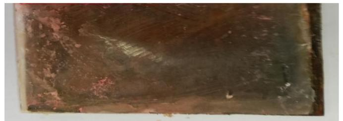
Figure (13): Blank epoxy coated sample after 17 days of NaOH exposure
