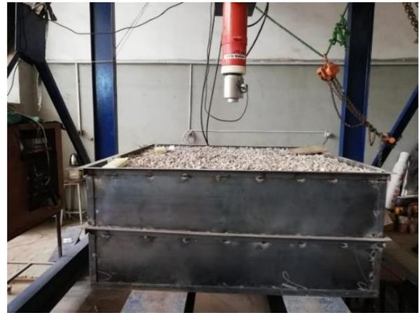
**Figure 3: The steel container filled with subbase layers.**
