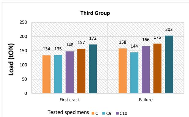
Figure 13: Loading test for third group samples
