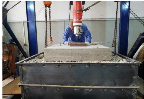
**Figure 2: The specimen was placed in the middle of container and the steel plate was placed in its center.**
