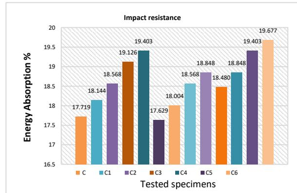
**Figure 10: Effect of waste rubber on energy absorption.**
