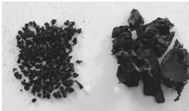
**Figure 1: Grinded rubber and shredded rubber**
