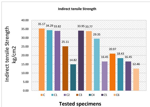
**Figure 8: Effect of rubber waste on indirect tensile strength**
