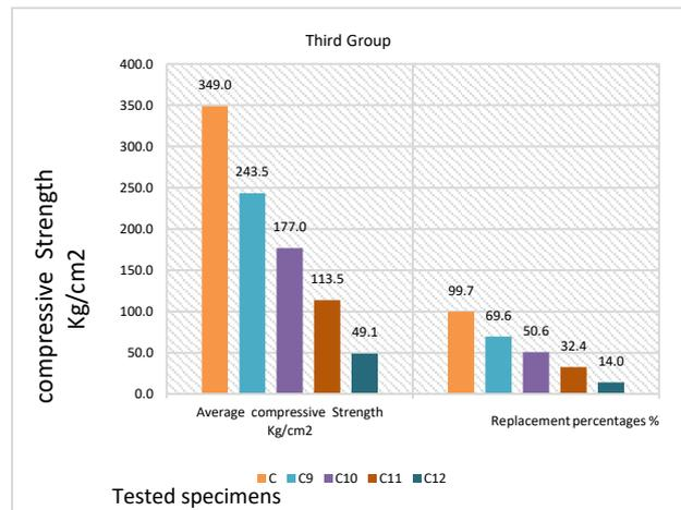
**Figure 6: Compression strength at different replacement percentages of rubber as fine aggregates.**
