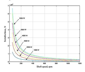
Figure 3: The shaft rotational speeds Vs the forces acting on the shaft.
