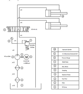
Figure 10: A configuration of hydraulic oil system.
