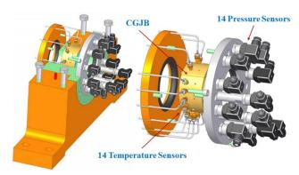
Figure 7: Modifications in regard to the pressure transmitters and temperature sensors.
