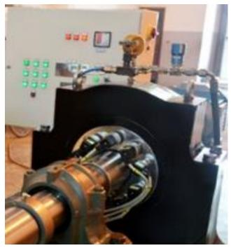
Figure 1: Journal bearing test rig structure. [1]
