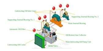
Figure 12: lubricating oil system.
