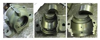
Figure 8: The modified supporting journal bearing
