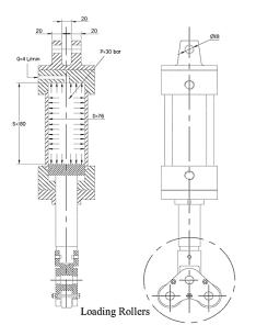
Figure 9: Hydraulic pistons with loading rollers.
