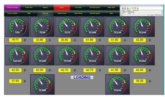
Figure 23: Oil film temperature distribution display page.
