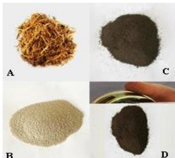
**Figure 1: Photographs of (A) sugarcane bagasse, (B) bagasse pith (BP), (C) magnetic bagasse pith (MBP), (D) MBP attracted to magnet.**
