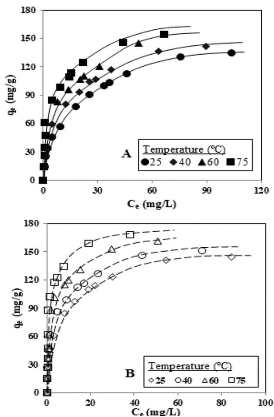
Figure 5: Equilibrium isotherms for adsorption of MB: (A) onto BP and, (B) onto MBP.
