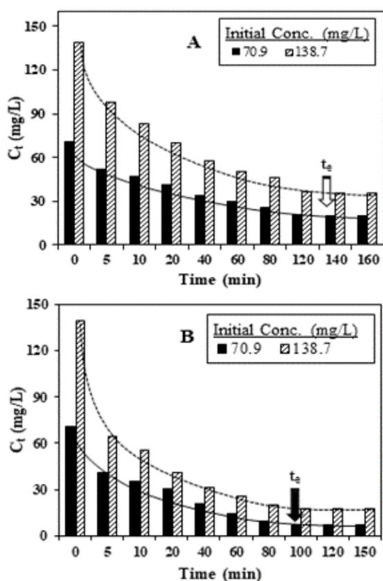
Figure 4: Contact time for adsorption of MB: (A) for BP and, (B) for MBP.
