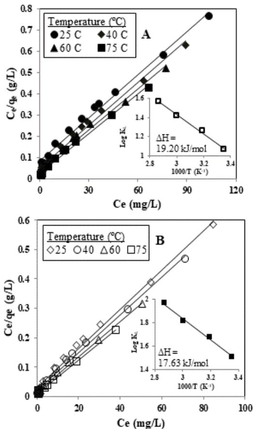
Figure 6: Langmuir plots for MB: (A) onto BP and, (B) onto MBP
