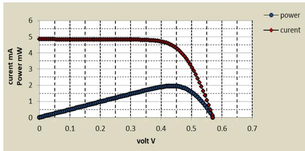
**Figure: 8  $TiO_2$  cell behavior when using N.719 dye**
