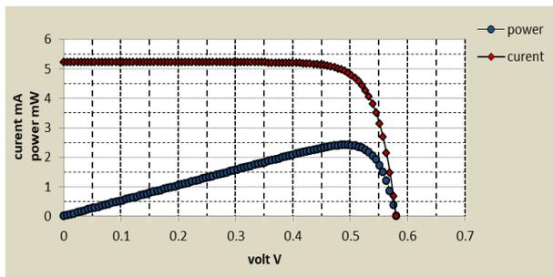
**Figure 10: Cell behavior of TiO<sub>2</sub> as a semiconductor with dye concentration 50%**
