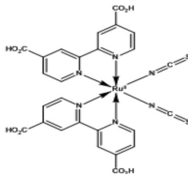
Figure 4: Structure of N3 dye molecule (N719): (Bu<sub>4</sub>N)<sub>2</sub>[Ru(dcbpyH)<sub>2</sub>(NCS)<sub>2</sub>] (Figure 5)
