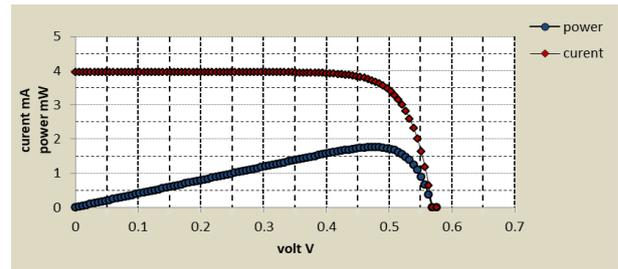
**Figure: 9  $TiO_2$  cell behavior when using N749 Black Dye**
