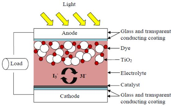
**Figure 1: Schematic of the energy flow in a dye-sensitized solar cell**
