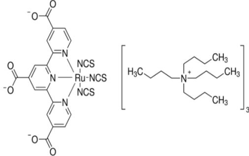
**Figure 6: Structure of N749 Black Dye [11]**
