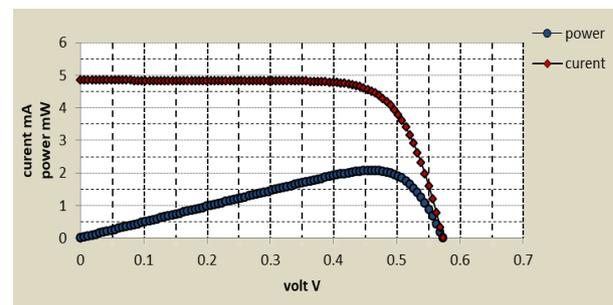
**Figure 11: Cell behavior of TiO<sub>2</sub> as a semiconductor with dye concentration 30%**
