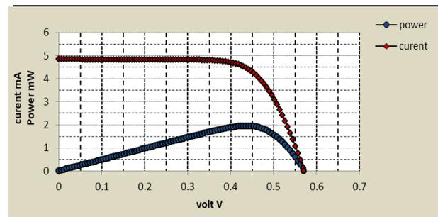
**Figure 7: TiO<sub>2</sub> cell behavior when using N.3 dye**
