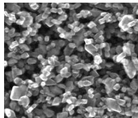
Figure 3: SEM micrograph of a nanocrystalline TiO<sub>2</sub> film (viewed from the top)
