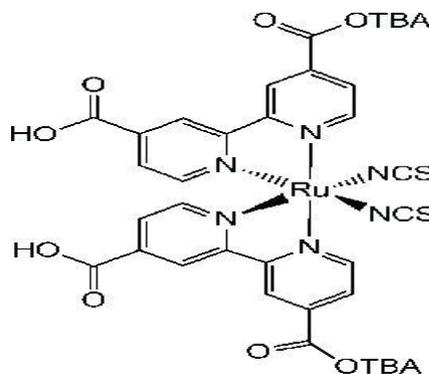
**Figure 5: Structure of N719 Dye [10]**
