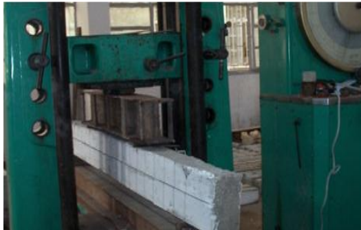
Figure. 2: Setup of beam test
