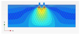
Figure 5: Lateral strain distribution for S1
