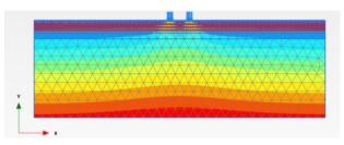
Figure 8: Vertical stress distribution for S10
