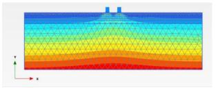
Figure 7: Vertical stress distribution for S1
