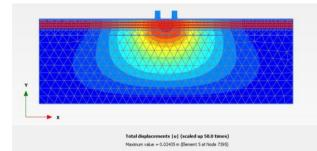
**Figure 4: Settlement distribution for research model** The obtained results of maximum settlement are indicated in table 6.
