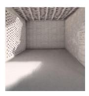
Figure 20: Examples of laser-cut fenestration pattern scale models and their perspective shadow studies in natural light.
