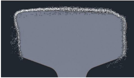
Figure 13: Solid work for a cross-sectional of the worn railhead
