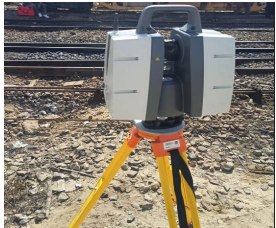
Figure 9: P40 3D Laser Scanner
