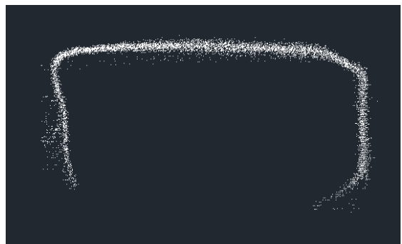
Figure 12: Cross-sectional of the worn railhead
