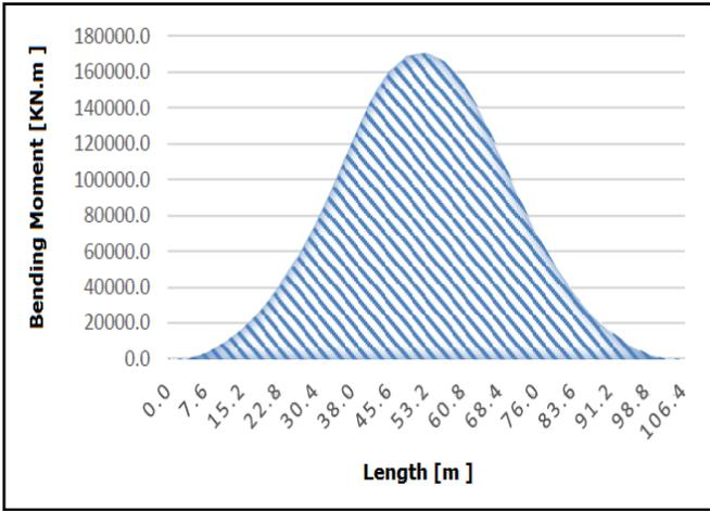
Fig. 10: Longitudinal Bending Moment Diagram
