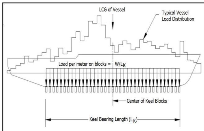
**Fig. 2: Load per meter run of the docked vessel [3]**
