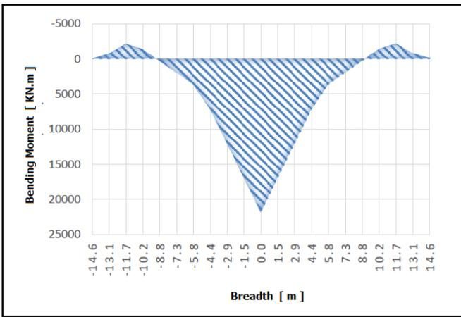
Fig. 11: Transverse Bending Moment Diagram
