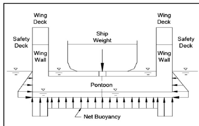
**Fig.1: Floating dry dock components [1]**
