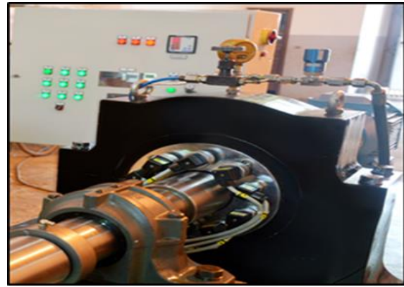
Figure 1: The Journal Bearing Test Rig (JBTR) by which the experiment was conducted
