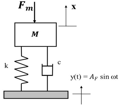
Figure 2 Equivalent model of the cantilever beam harvester.
