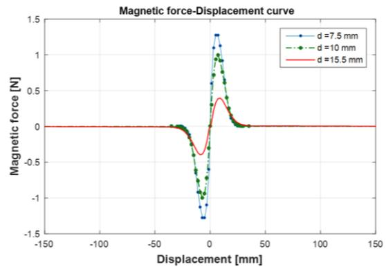
Figure 3 Magnetic force versus displacement at different gaps ( $d= 7.5$  mm ,  $d=10$  mm, and  $d=15.5$  mm ) measured experimentally by Hadidi et.al [27].
