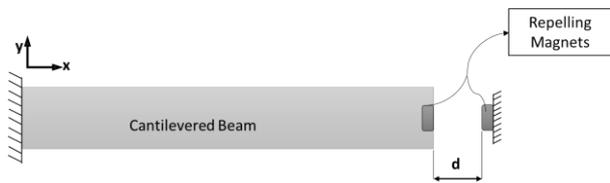
Figure 1 Schematic drawing of the nonlinear energy harvester
