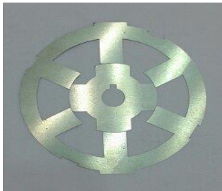
Figure 1. Cross section of One Lamination 6/4 SRM
