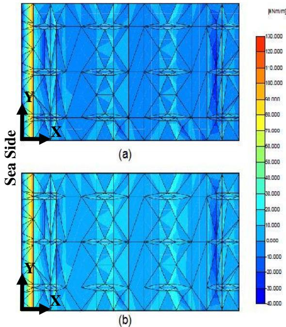
**Figure 17: Bending moment in X direction for deck slab; (a) Case (-22, 80), (b) Case (-22, 120).**
