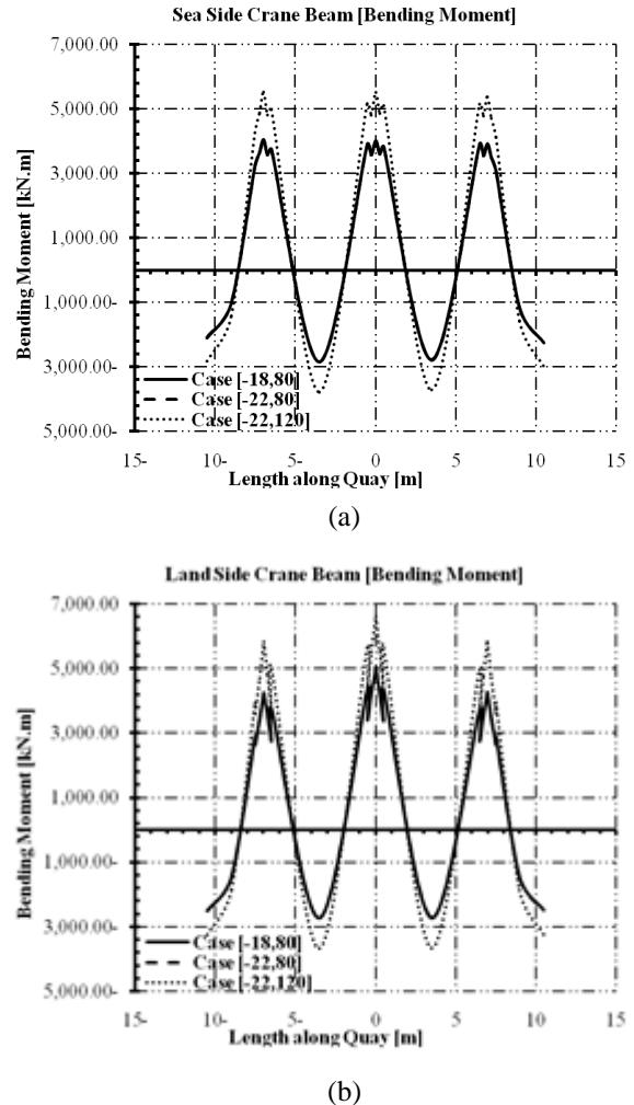
**Figure 15: Bending moment of crane beams; (a) Sea side crane beam, (b) Land side crane beam.**
