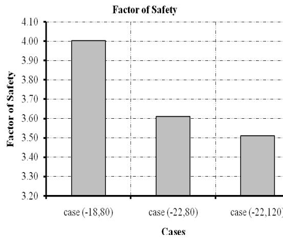
**Figure 18:  $\phi - c$  reduction factor of safety for three cases.**
