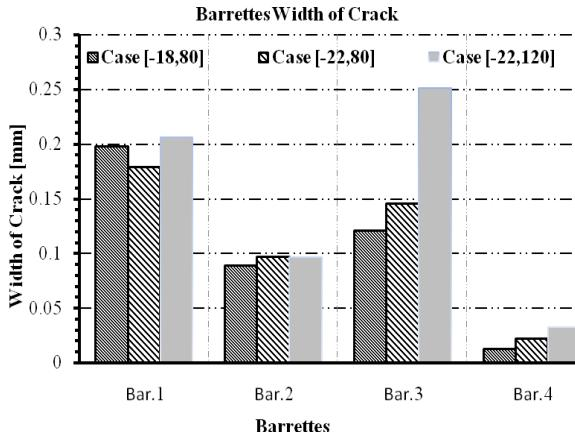
**Figure 13: Width of crack for all barrettes due to the three cases.**
