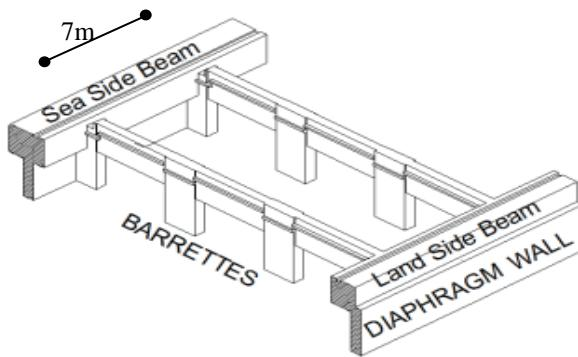
**Figure 4: Quay wall beams alignment.**
