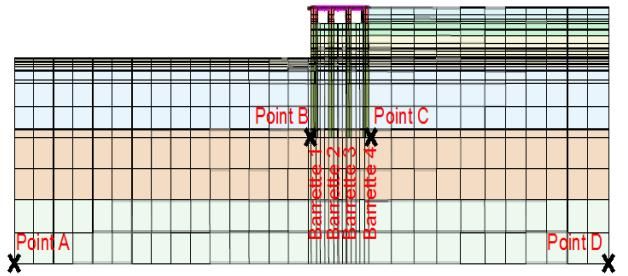
**Figure 6: Finite element mesh of the quay wall.**
