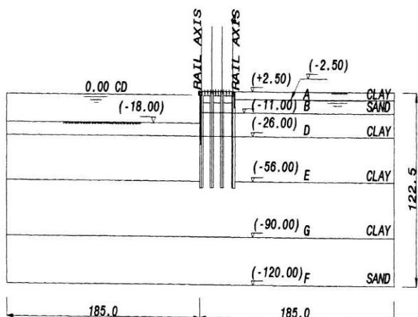
**Figure 5: Geometry of the analyzed model.**
