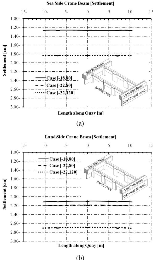
**Figure 14: Vertical settlement of crane beams; (a) Sea side crane beam, (b) Land side crane beam.**
