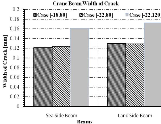
**Figure 16: Width of crack for crane beams due to the three cases.**
