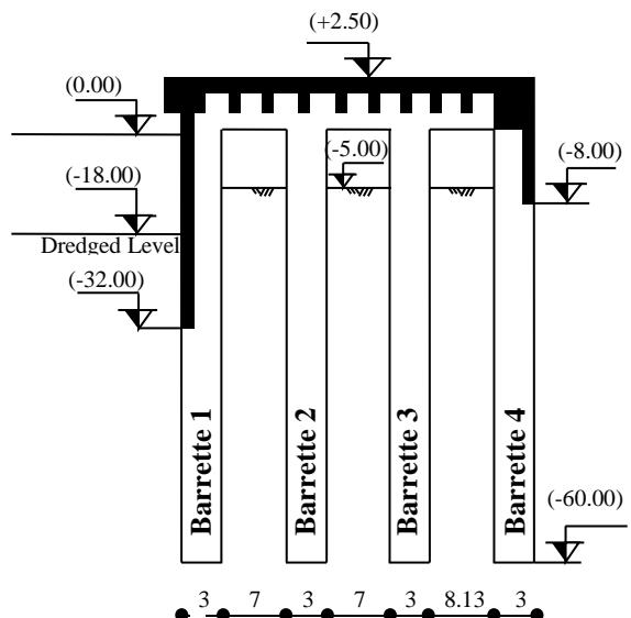
**Figure 3: Quay wall cross section.**
