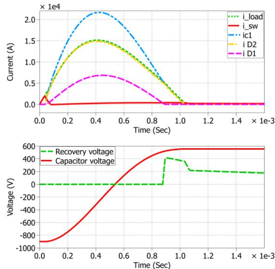
Fig. 8: Current and voltage wav-forms for HCLID with ZnO at 90 ele. degree inception angle.
