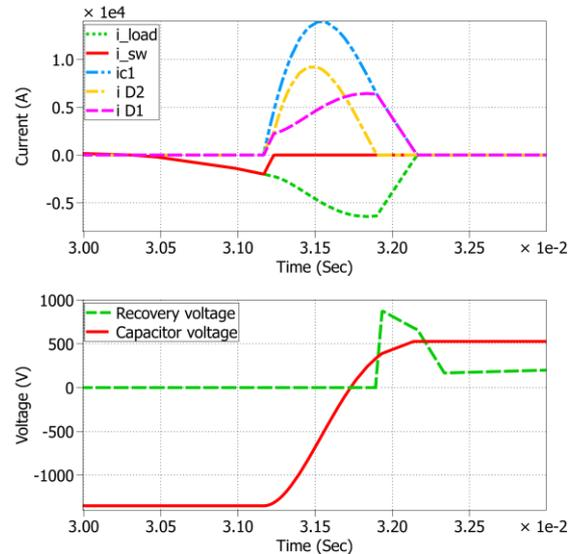
Fig. 6: Current and voltage wav-forms for HCLID without ZnO at 170 ele. degree inception angle.
