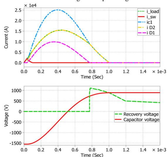
Fig. 5: Current and voltage wav-forms for HCLID without ZnO at 90 ele. degree inception angle.
