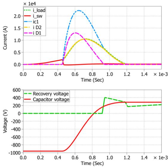
Fig. 7: Current and voltage wav-forms for HCLID with ZnO at 0 ele. degree inception angle.
