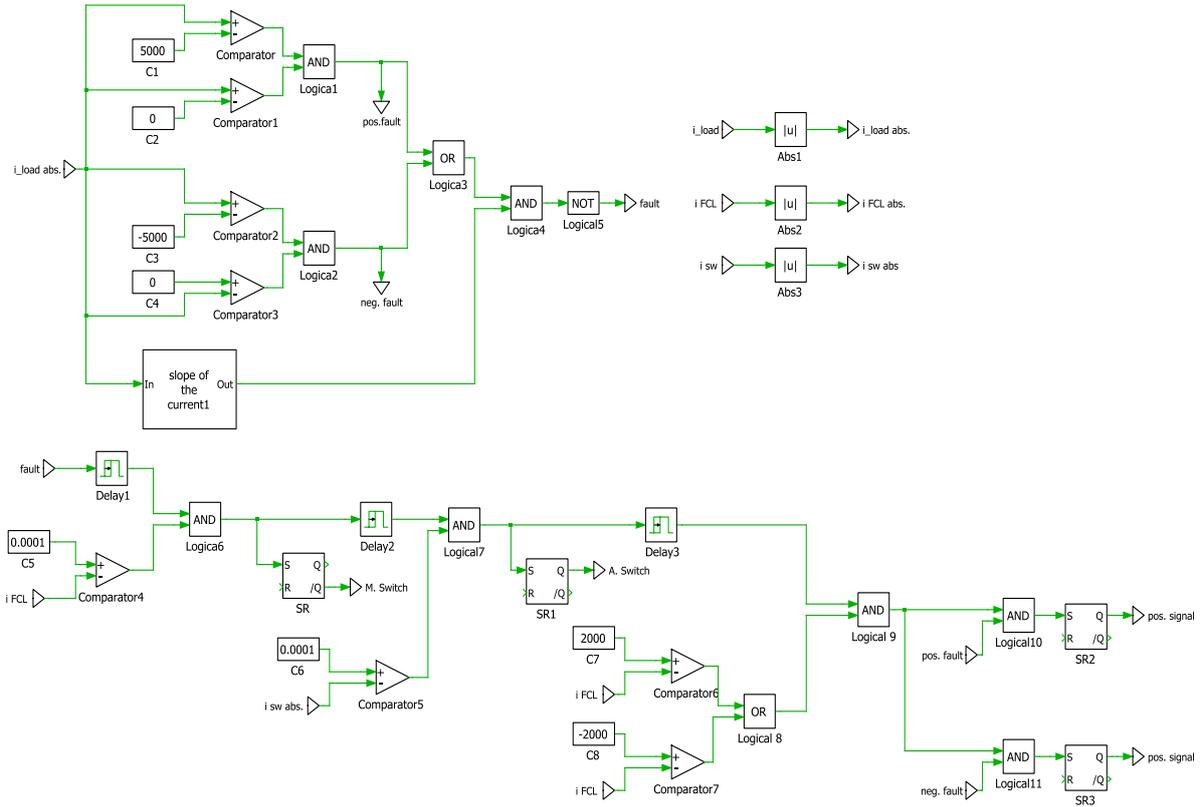
Fig. 2: Control algorithm implemented in PLECS program
