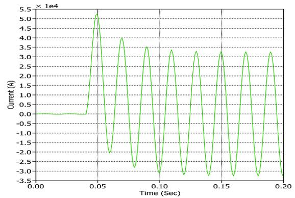
Fig. 3: Prospective fault current
