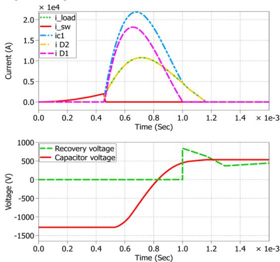
Fig.4: Current and voltage wav-forms for HCLID without ZnO at 0 ele. degree inception angle.
