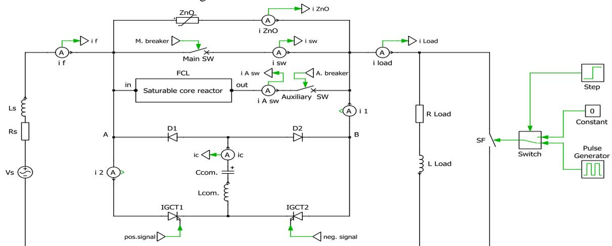
Fig. 1: HCLID circuit configuration
