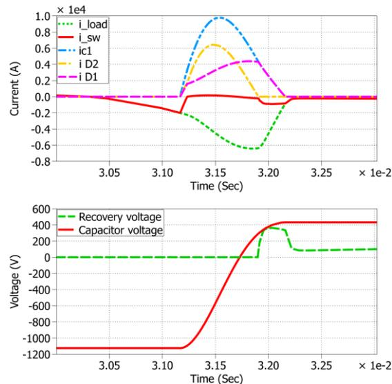
Fig. 9: Current and voltage wav-forms for HCLID with ZnO at 170 ele. degree inception angle.
