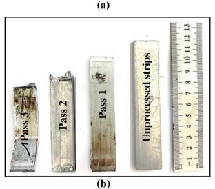
Figure 1: (a) the experimental set-up for the ECAP process and (b) unprocessed and ECAP processed samples (after 1, 2 and 3 passes).
