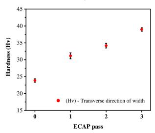
Figure 10: Average hardness and standard deviations (error bar) of 1050-aluminum samples of the annealed before and after ECAP up to 1<sup>st</sup>, 2<sup>nd</sup>, and 3<sup>rd</sup> passes.
