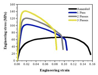
Figure 6: Engineering stress-strain curve of 1050-aluminum of before and after the ECAP processed samples.
