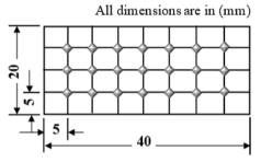
Figure 3: Schematic diagram showing the longitudinal direction in width for indentation locations of hardness for the annealed 1050-aluminum sample before and after ECAP process.
