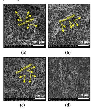
Figure 8: Tensile fractured surfaces of 1050-aluminum before and after the ECAP process: (a) 0 pass, (b) 1 pass, (c) 2 passes and (d) 3 passes.
