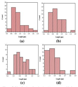
Figure 5: Distribution of grain size; (a) unprocessed before ECAP, and (b) 1 pass, (c) 2 passes, (d) 3 passes of ECAP processed samples.
