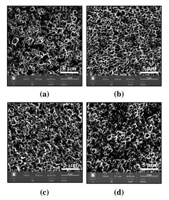
Figure 4: The scanning electron microscopy (SEM) observations: (a) before ECAP, (b) after the first pass, (c) after the second pass and (d) after the third pass of ECAP process.
