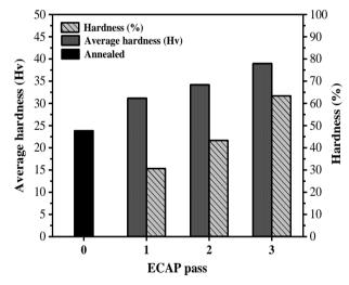
Figure 9: Hardness and hardness percentage in the longitudinal direction of width before and ECAP passes of 1050-aluminum samples.
