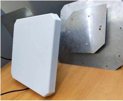
Figure 14: Photo of the fabricated antenna with a PETG cover.
