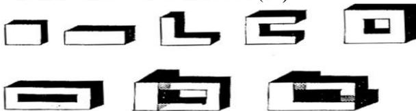
Fig (16) Effect of Building Form on Shadow Formation Scale, beside the role of Courtyards and variation in building height on shadow formation. (6)
