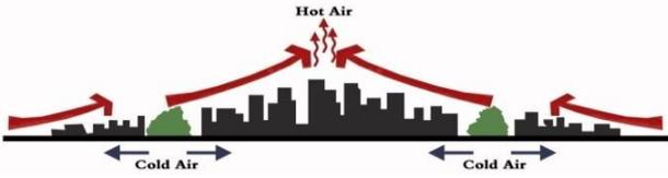
**Fig (10) Flow of Cold Air from public spaces and outskirts of the city to the City Center with condense buildings area.**
