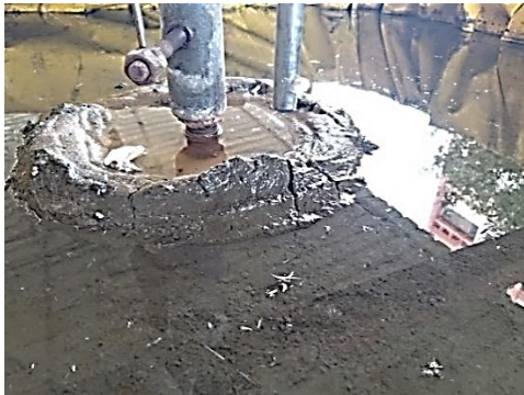
Figure 14: Settlement under footing for SR method
