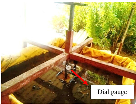
Figure 8: Final stage of scaled soil profile and test setup
