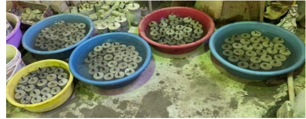
Figure 4: Concrete cylindrical specimens exposed to aggressive media.
