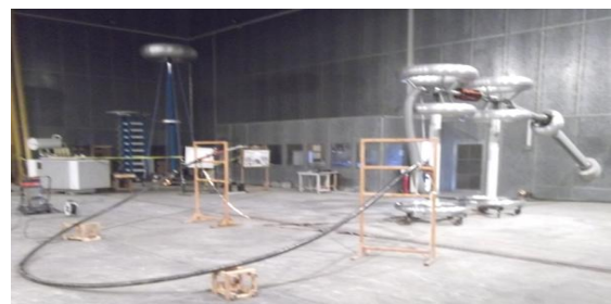
Figure 2: Test circuit inside shielded enclosure
