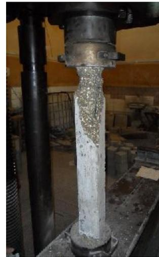
Fig.5 Original column failure
