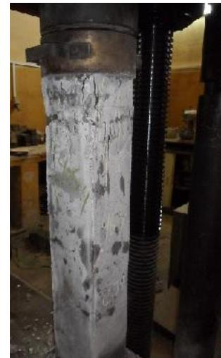
Fig.6 Jacket failure of group (A)
