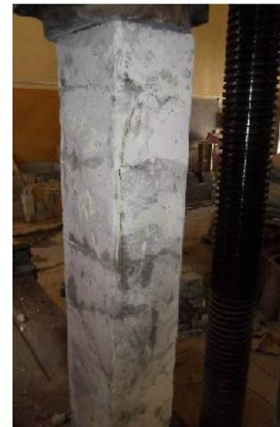
Fig.7 Jacket failure of group (B)
