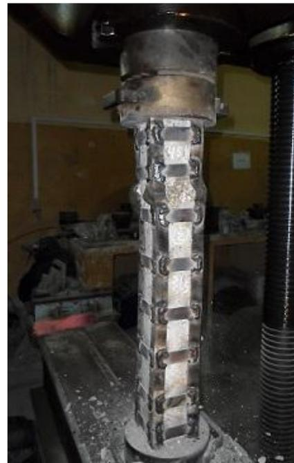
**Fig.11 Jacket failure of group (E)**
