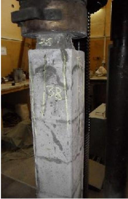
**Fig.8 Jacket failure of group (C)**
