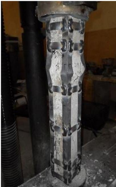
**Fig.9 Jacket failure of group (D)**
