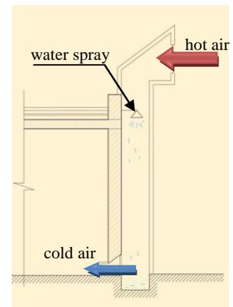
Figure 8 : Evaporative cooling system proposal
