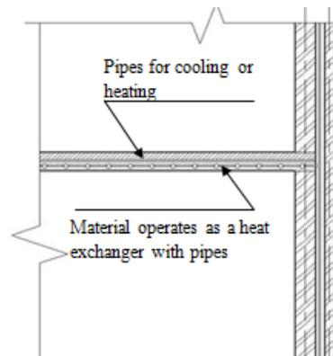
**Figure 12:** Pipes for cooling or heating
