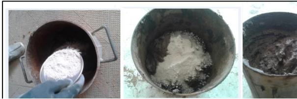
**Figure (1):** Mixing Soft Clay Soil and Quicklime.
