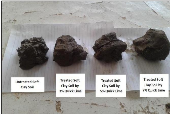
**Figure (2):** Comparing Untreated Soft Clay to Quicklime-Treated Clay after Initial Mixing with Different Percentage of Quicklime.
