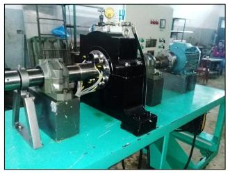
Figure 3: The Journal Bearing Test Rig "JBTR". [6]
