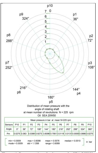
Figures 4: Representation of polar curve for SEA 20W50. 6.2 Polar pressure distribution curve for SEA 10W40 [6]
