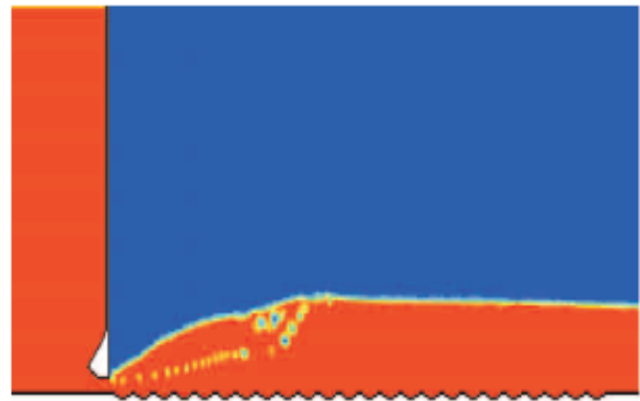
Figure 1 Simulation of free water surface by using VOF method.
